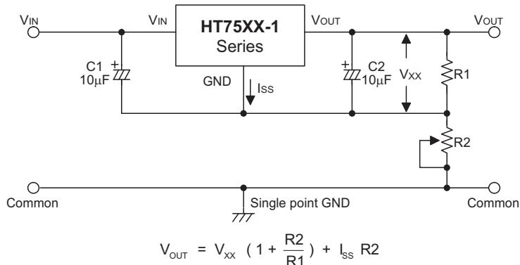
**Circuit for Increasing Output Voltage**
